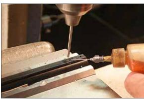
9. Lubricate & drill out both starter holes using a #31 bit. Re-drill the original hole if smaller than 6-48.
