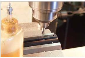
8. Drill two starter holes, the first .375" forward, and the second .750" forward, between centers.
