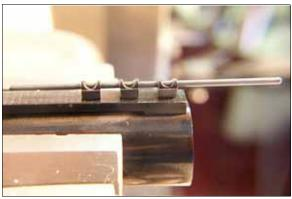
14. Use a length of 1/16th inch drill rod to confirm that all the beads line up correctly.
