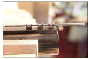
16. Again back off all beads less than a half turn from bottom and re-align all three beads with drill rod. Wait for the Lock-tite to set.
