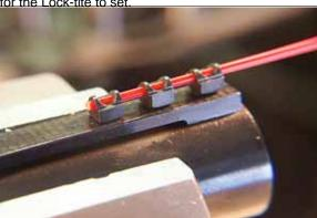
17. Insert the fiber-optic rod choice so that roughly 1/16th inch protrudes past the front bead. The longer the protrusion, the larger the resulting bulb.
