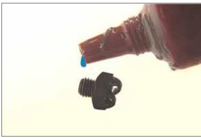
15. In turn, remove each bead, put a small drop of **blue** Lock-tite on the threads, and re-install the bead.
