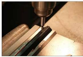
6. Locate the edge of the rib & move half the rib width to locate center.
