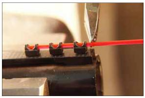
19. Use side cutters to trim the fiber-optic rod roughly 1/16th inch past the end of the rear bead.
