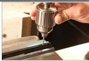
10. Lubricate & use a 6-48 starter tap to hand start all three holes. Use the mill to ensure the taps are started vertically. *Avoid denting the barrel*.
