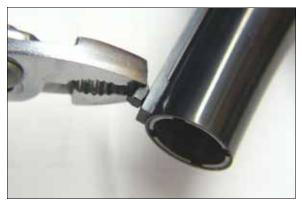
1. Detach the barrel & remove the front bead.
