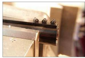
12. Thread in all beads in by hand until each bottoms out. Visually confirm each is at the same height.
