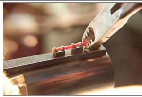
To quickly change sight color, cut the rod between the beads, remove the old rod, & repeat steps 17-21 to install a new rod color. Rod change takes about two minutes & requires only a cutter and lighter.
