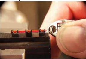
20. Briefly touch a lighter to the rear of the fiber-optic rod, forming the rear bulb and locking the rod in place between the front and rear beads.
