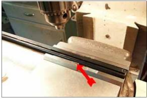
2. Clamp the barrel in the mill vise with minimum pressure to prevent crush. Pad & shim the barrel.
