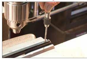
11. Finish hand-tapping with a 6-48 bottom tap. *Avoid denting the barrel.*
